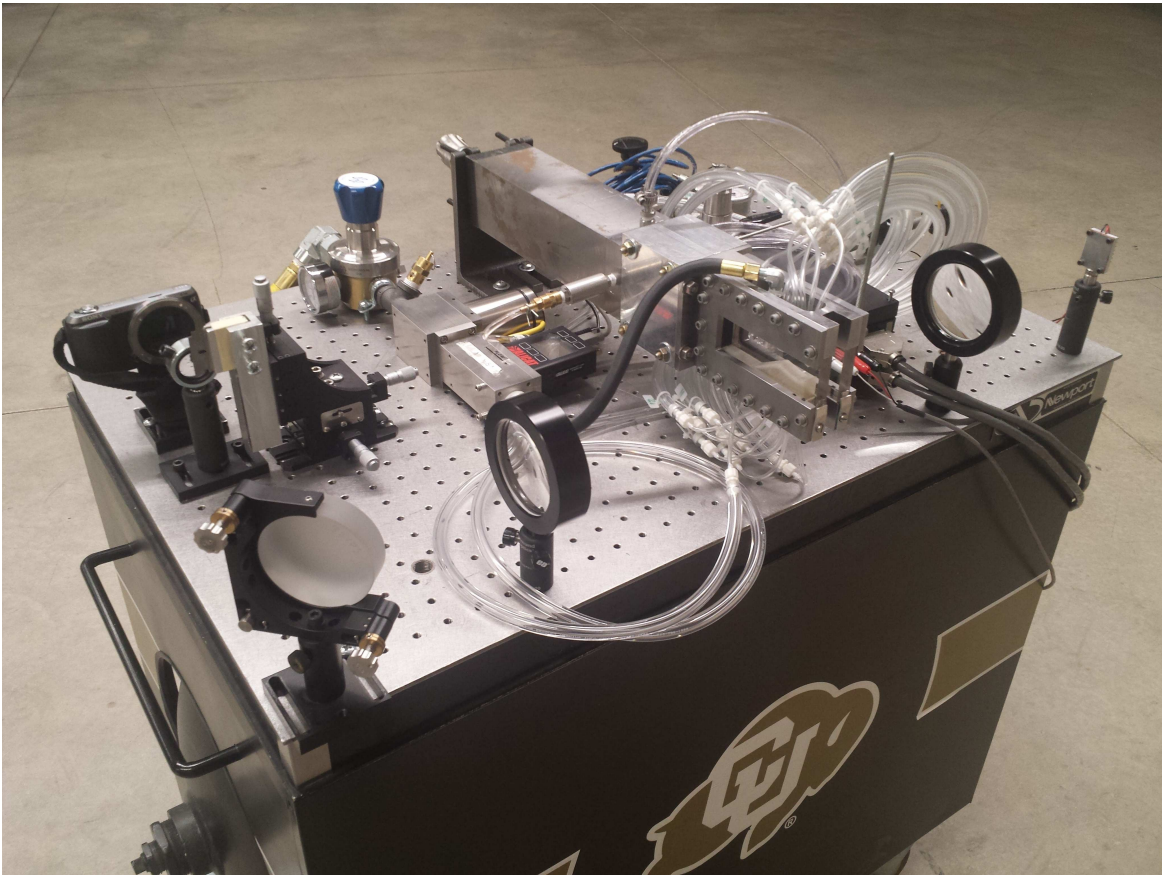
Figure A.1: View of test setup including diffuser, test section, and schlieren system.
